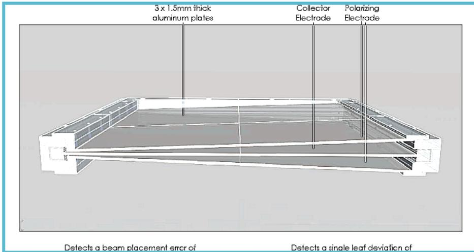
**Large area ionization chamber** with a gradient in the electrode plate separation (in the axis of MLC motion)
