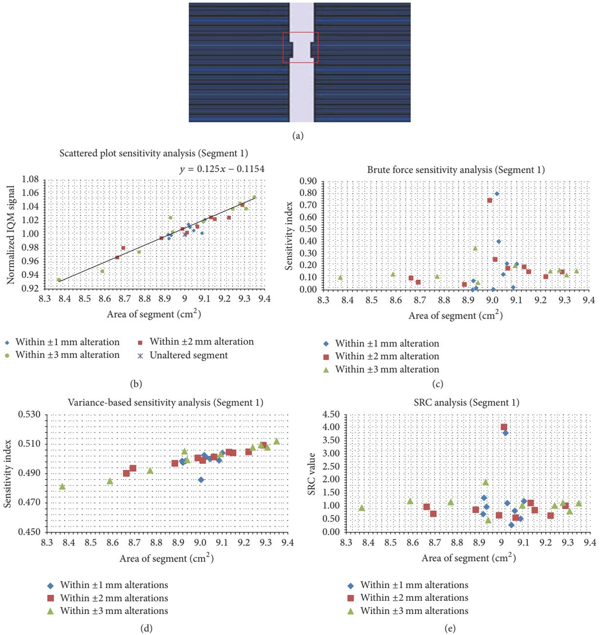
FIGURE 5: Sensitivity analysis results for the  $3 \times 3 \text{ cm}^2$  segment. Panel (a) shows the unaltered segment; panel (b) shows the scatter plot; panels (c), (d), and (e) show the brute force, variance-based, and standard regression coefficient results, respectively.
