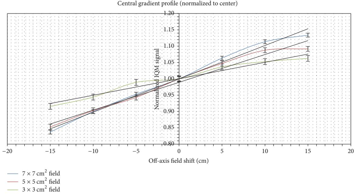
FIGURE 4: Sensitivity factor along the IQM CM gradient for 3 × 3, 5 × 5, and 7 × 7 cm<sup>2</sup> fields (trend gradients are 0.005, 0.009, and 0.010).
