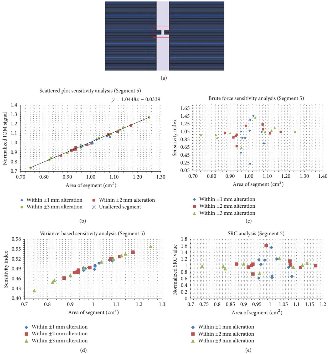
FIGURE 9: The same data as in Figure 4, but for the irregular segment with an area of  $1.0 \text{ cm}^2$ . Panel (a) shows the unaltered segment; panel (b) shows the scatter plots; panels (c), (d), and (e) show the brute force, variance-based, and standard regression coefficient results, respectively.
