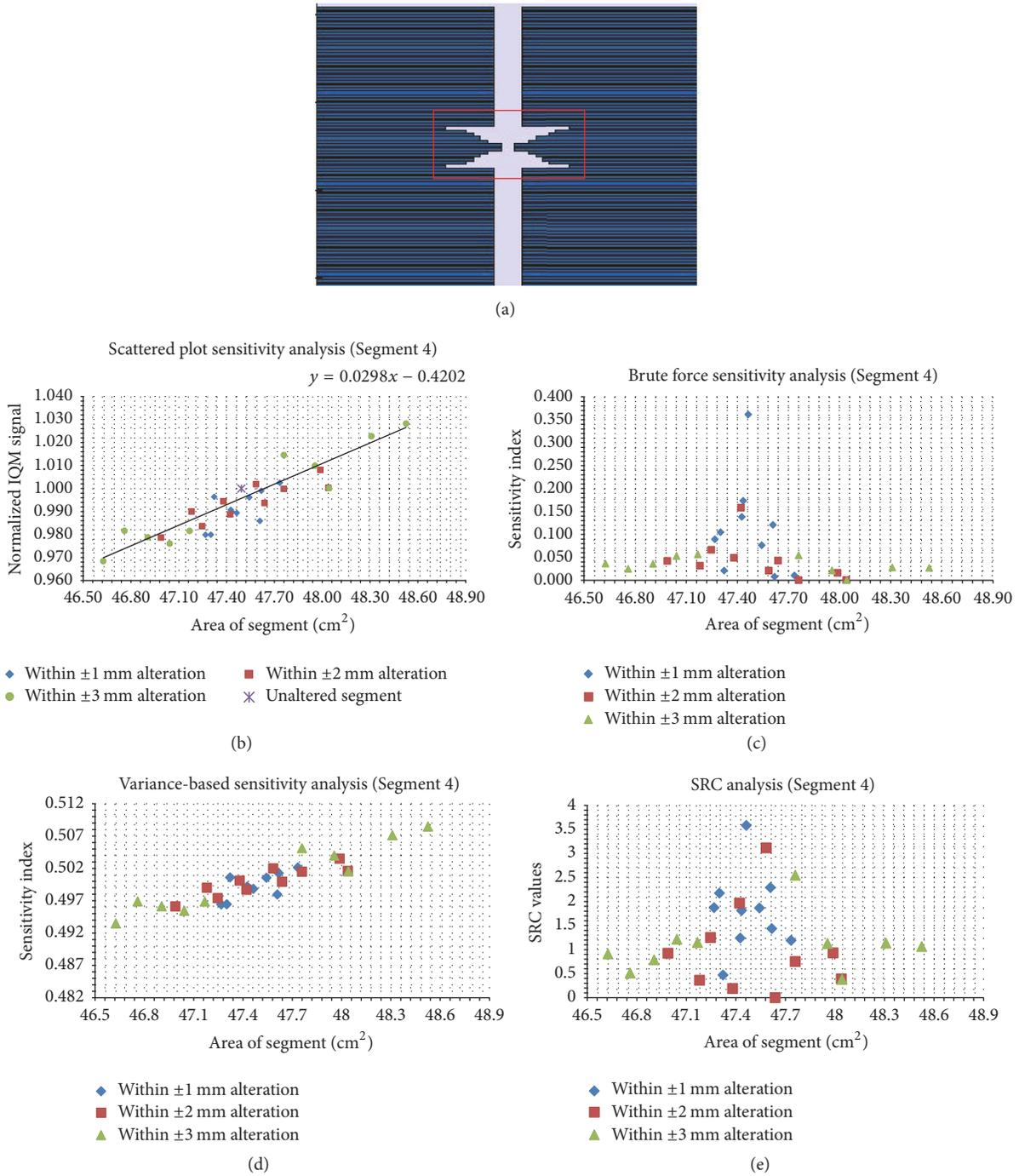
FIGURE 8: The same data as in Figure 4, but for the irregular segment with SA of 47.49 cm<sup>2</sup>. Panel (a) shows the unaltered segment; panel (b) shows the scatter plots; panels (c), (d), and (e) show the brute force, variance-based, and standard regression coefficient results, respectively.
