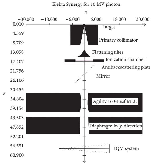
FIGURE 2: Setup of the IQM geometry located 4.5 cm below the Y-diaphragm for  $10 \times 10$  cm<sup>2</sup> field.
