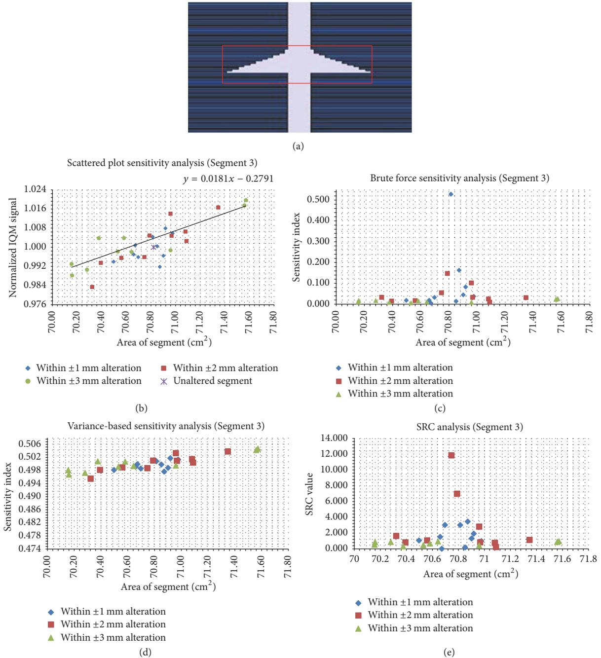
FIGURE 7: The same data as in Figure 6, but for the irregular segment with an area of 70.82 cm<sup>2</sup>. Panel (a) shows the unaltered segment; panel (b) shows the scatter plots; panels (c), (d), and (e) show the brute force, variance-based, and standard regression coefficient results, respectively.
