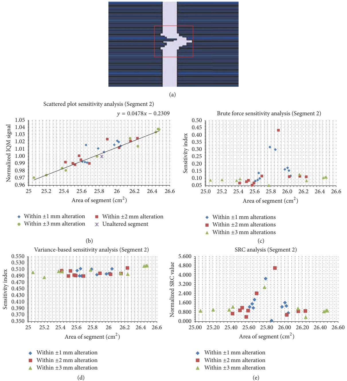
FIGURE 6: Sensitivity analysis results for an irregular segment ( $SA = 25.83 \text{ cm}^2$ ). Panel (a) shows the unaltered segment; panel (b) shows the scatter plots; panels (c), (d), and (e) show the brute force, variance-based, and standard regression coefficient results, respectively.
