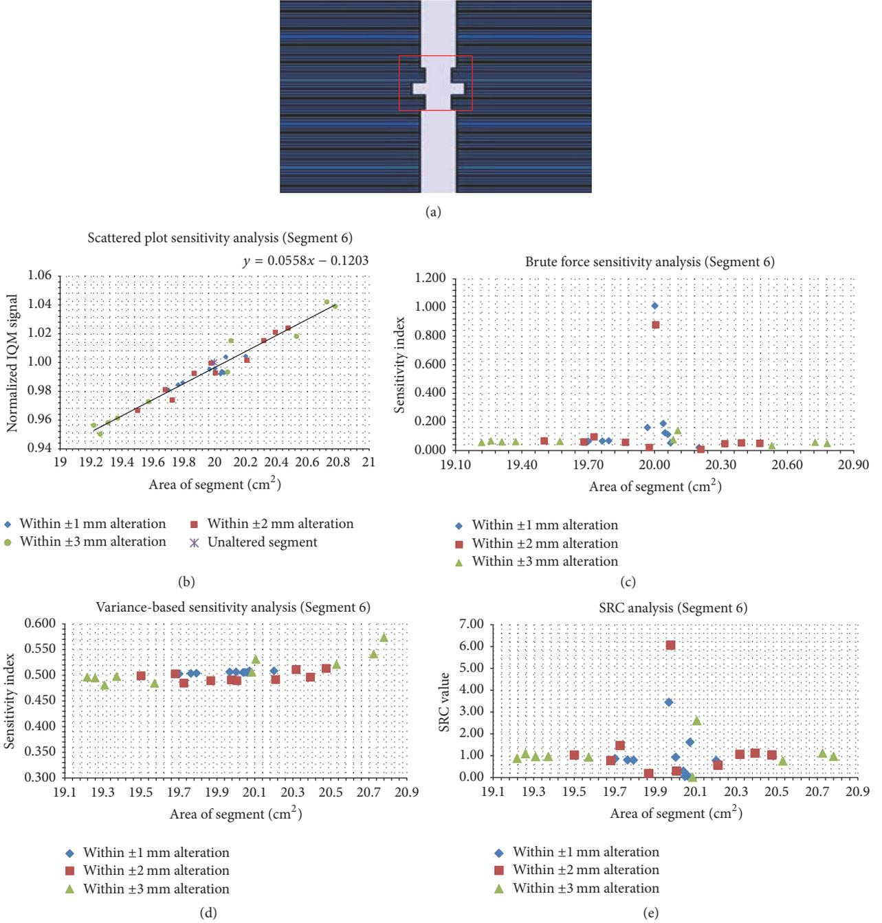
FIGURE 10: Sensitivity analysis results for an irregular segment (SA = 19.99 cm<sup>2</sup>). Panel (a) shows the unaltered segment; panel (b) shows the scatter plots; panels (c), (d), and (e) show the brute force, variance-based, and standard regression coefficient results, respectively.
